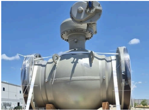
ACTUATED BALL VALVE, BLOCKED UNDER THE BODY
